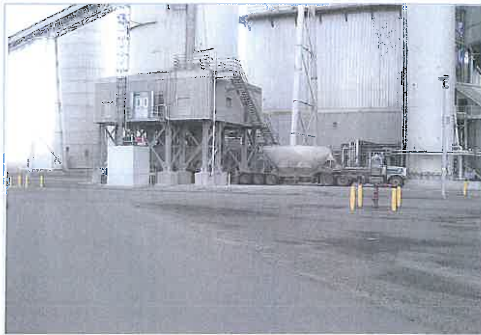
Figure 7 – Loading dry fly ash to bulk pneumatic trailer for transport offsite
