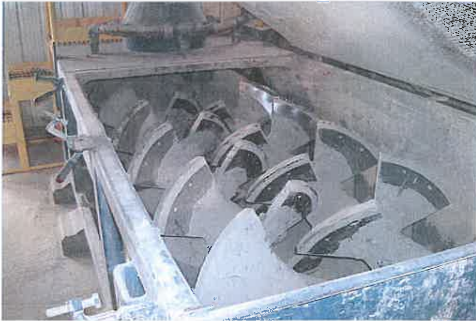
Figure 5 – Pugmill for adding and mixing water to dry fly ash
